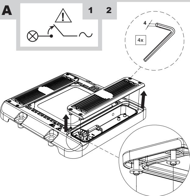
Note: Screws are loose in the lid. The retaining washers prevent them from falling out.
