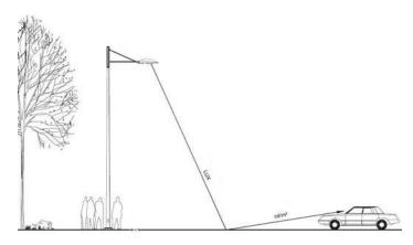
Surfaces with different reflecting properties will have the same illuminance, but different luminance. The main criterion requested by the standard for road lighting applications is the luminance of the road surface. The good knowledge of the light reflection characteristics of the road pavements is consequently of main importance for achieving an accurate lighting design.
