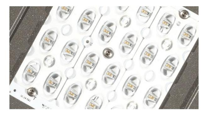
The LensoFlex®3 photometric engine, like LensoFlex®2, is based upon the addition principle of photometric distribution; each LED is associated with a specific lens that generates the complete photometric distribution of the luminaire. The main difference is the material used for the lenses.
